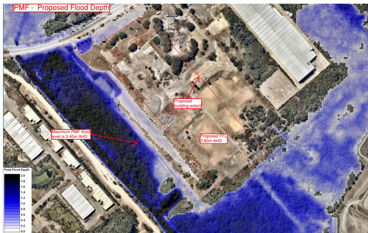
Figure 12 – Post Development PMF Depth
